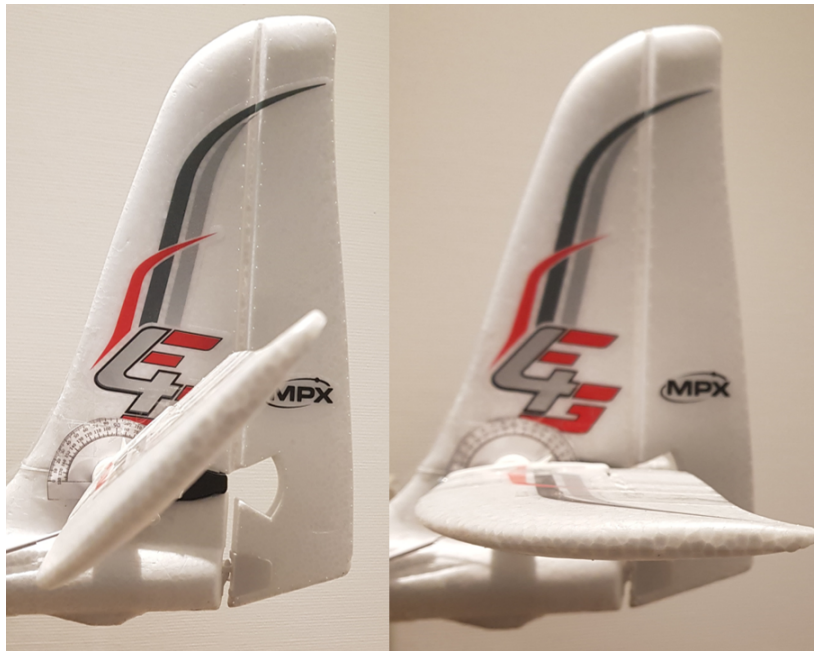
Figure 3.2: The left picture shows the elevator with the maximum deflection of approx. 50^\circ . The right one shows the neutral position.
